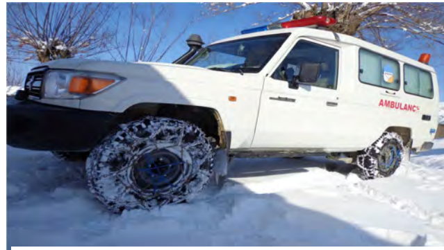
Above: The MDF ambulance equipped with snow chains to ensure a safe operation in snowy conditions.
